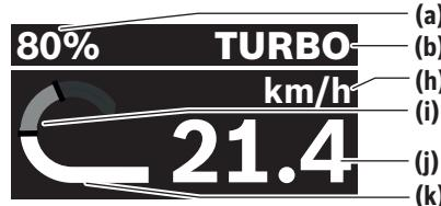
(a) State of charge of eBike battery (can be configured)
